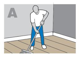
A Ensure that the subfloor is reasonably level, sound, dry and free from dust, grease or other contaminants.
