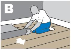
**B Whisper** underlay can be laid either side up but must be laid at right angles to any existing floorboards. When installing **Whisper** underlay allow for a 5cm excess to run up the walls.
